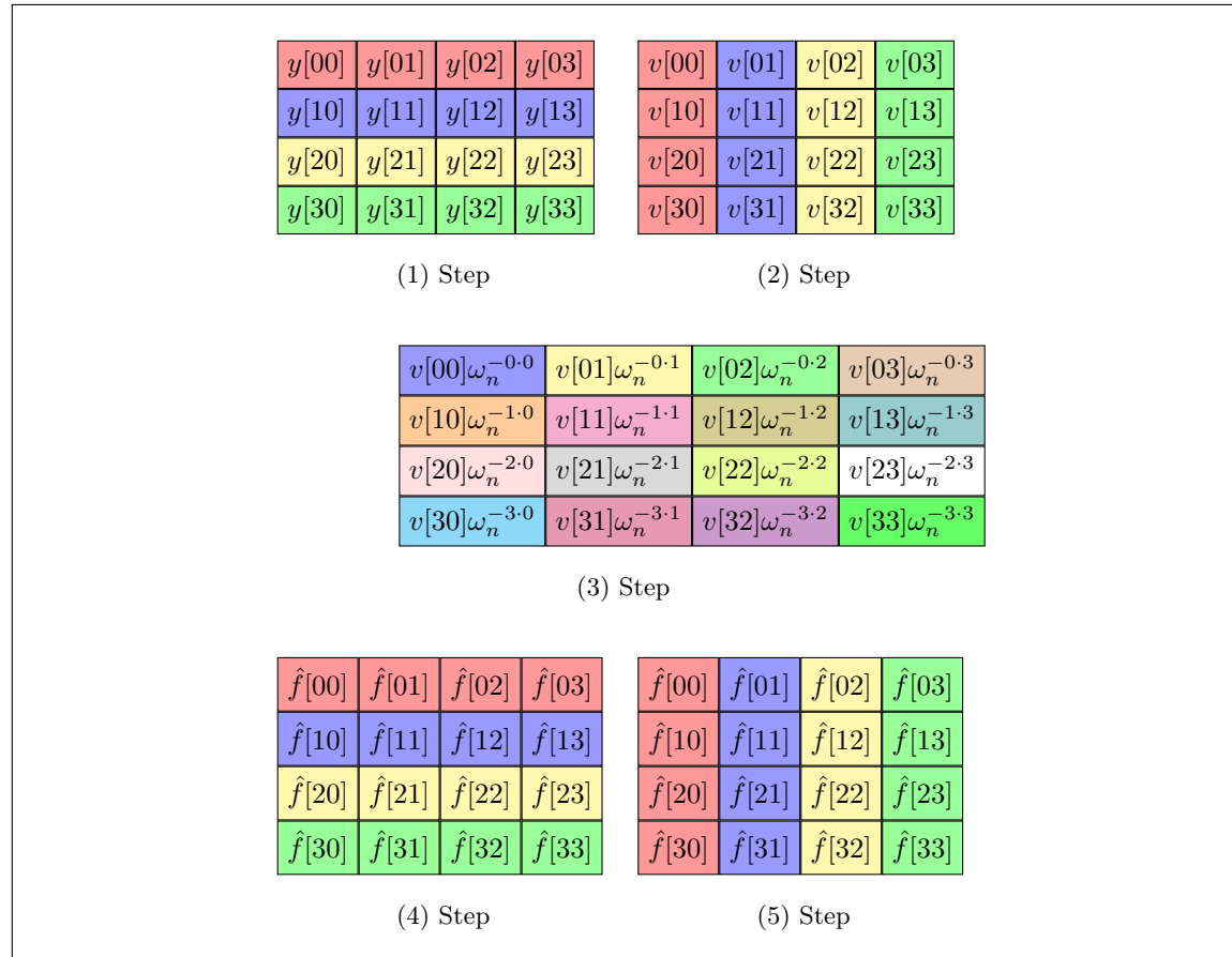
Figure 3: Schematic procedure of a Cooley-Tukey FFT
